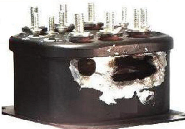
Fig. 12. Failed relay due to tin vapor arcing.
